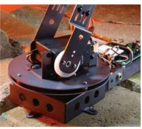
The completed SG6 arm has a sturdy pivot table to which the arm is securely mounted. In the background, the Parallax Board of Education prototyping board is visible. The "grilled" plate at the top of the arm is a sensor bracket.
